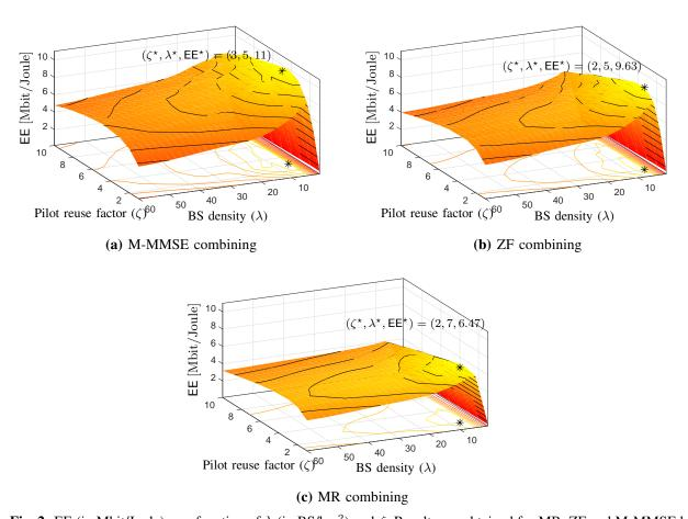
Fig. 2: EE (in Mbit/Joule) as a function of  $\lambda$  (in BS/km<sup>2</sup>) and  $\zeta$ . Results are obtained for MR, ZF and M-MMSE by using Monte Carlo simulations within a Massive MIMO setting with M=100 and K=10. The global optimum is star-marked for which the corresponding values of  $\zeta$ ,  $\lambda$  and EE are also reported.
