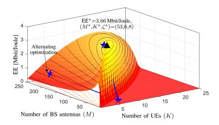
Fig. 5: EE (in Mbit/Joule) of ZF as a function of M and K, for fixed  $\gamma = 3$ ,  $\lambda = 10 \text{ BS/km}^2$ ,  $\text{SNR}_0 = 5 \text{ dB}$  and  $\text{SNR}_p = 15 \text{ dB}$ . The global optimum obtained from Monte Carlo simulations is indicated with a black triangle. This is compared to the optimum achieved by using Algorithm 1 (blue star).
