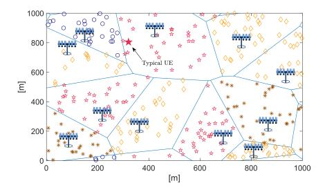
Fig. 1: Deployment of a cellular network with BSs drawn from a H-PPP  $\Phi_{\lambda}$ , each one serving K randomly located UEs. The "typical" UE k in cell j is highlighted. The UEs of different cells sharing the same pilot subset  $\Phi_{l}$  are depicted with the same marker and color. We consider  $A=1\,\mathrm{km^2}$ ,  $\lambda=16$ ,  $\zeta=4$  and K=30.
