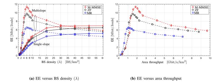
Fig. 3: EE (in Mbit/Joule) as a function of (a)  $\lambda$  (in BS/km<sup>2</sup>) and (b) Area Throughput in (in Gbit/s/km<sup>2</sup>) for the optimal numerical  $\zeta^*$ . Results are obtained from Monte Carlo simulations for MR, ZF and M-MMSE combiners within a Massive MIMO setting with M=100 and K=10. In Fig. 3a, both single-slope and multislope path loss models are considered while in Fig. 3b only the multislope is considered.
